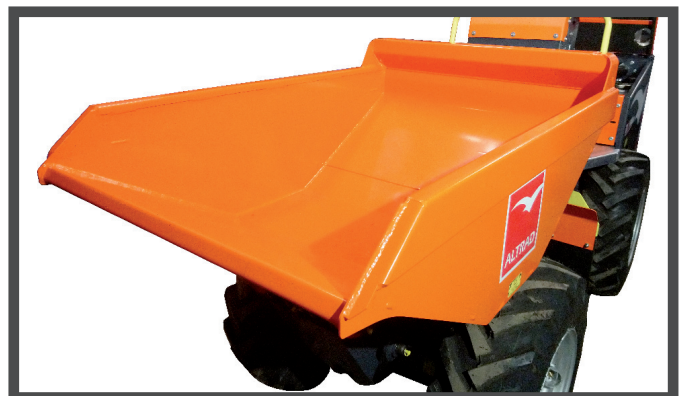
ROBUST, EASY-CLEAN 1000KG CAPACITY SKIP FULLY RETURNED EDGES TO PREVENT DIRT INGRESS
