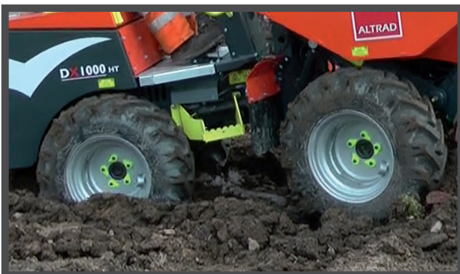
HIGH-QUALITY, ALL-TERRAIN TYRES WITH VALVE PROTECT GUARD & WHEEL NUT INDICATORS
